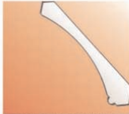
Harbor Classic Crown Slope= 44^{\circ} Bevel Angle = 29.42^{\circ} Miter Angle = 54.27^{\circ} Miter Saw Setting = 35.73^{\circ}
