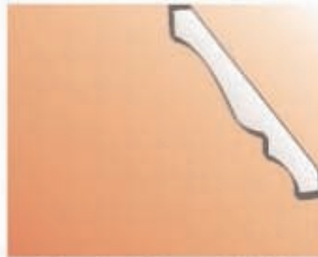
Classical Crown 3 5/8" Slope= 55^{\circ} Bevel Angle = 35.4^{\circ} Miter Angle = 60.16^{\circ} Miter Saw Setting = 29.84^{\circ}
