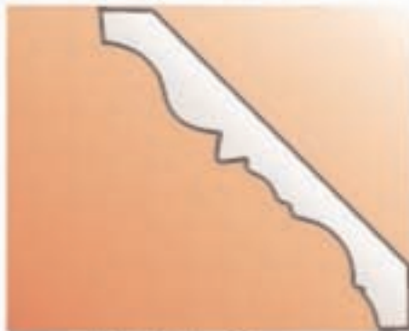
Victorian Crown Slope= 45^{\circ} Bevel Angle = 30^{\circ} Miter Angle = 54.74^{\circ} Miter Saw Setting = 35.26^{\circ}
