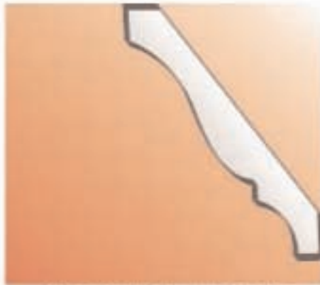
Classical Crown 4 5/8" Slope= 53^{\circ} Bevel Angle = 34.38^{\circ} Miter Angle = 58.96^{\circ} Miter Saw Setting = 31.04^{\circ}
